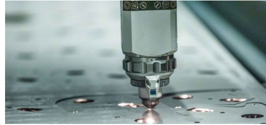
<p>When cutting stainless steel in the thickness range of three to 20 millimeters, DELO needs up to 70 percent less nitrogen with the HighSpeed Eco option.</p>
